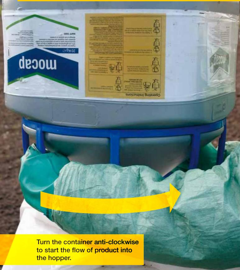
Turn the container anti-clockwise to start the flow of product into the hopper.
