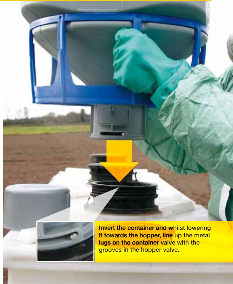
Invert the container and whilst lowering it towards the hopper, line up the metal lugs on the container valve with the grooves in the hopper valve.
