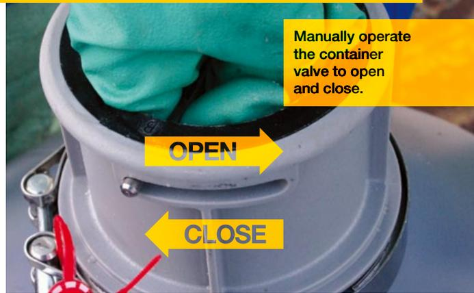
**Manually operate the container valve to open and close.**
