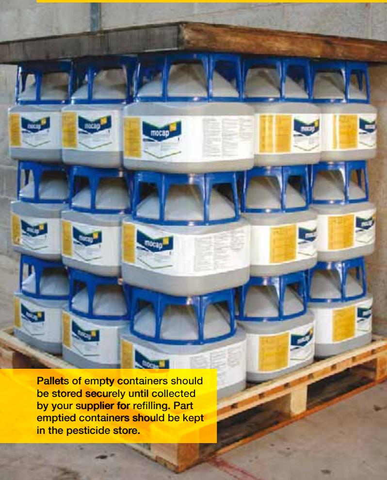
Pallets of empty containers should be stored securely until collected by your supplier for refilling. Part emptied containers should be kept in the pesticide store.
